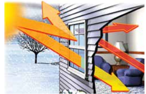
Winter Energy Savings: Low-E insulating glass helps reduce heat loss by reflecting warmth back into your home.
